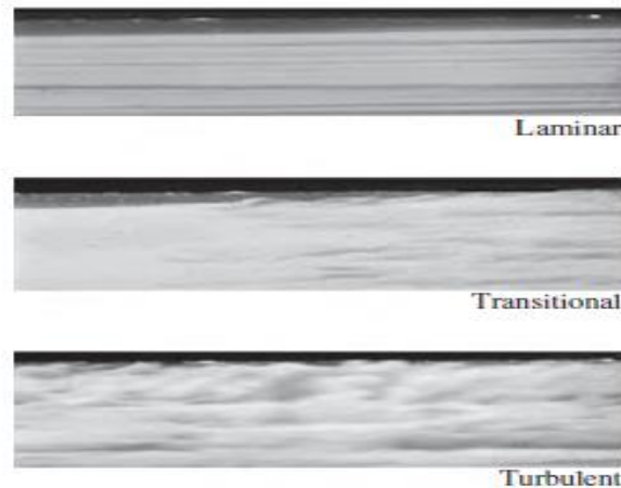
Figure 5. Laminar, Transitional and Turbulent flow characteristics. Source: (Çengel and Cimbala (2018).
